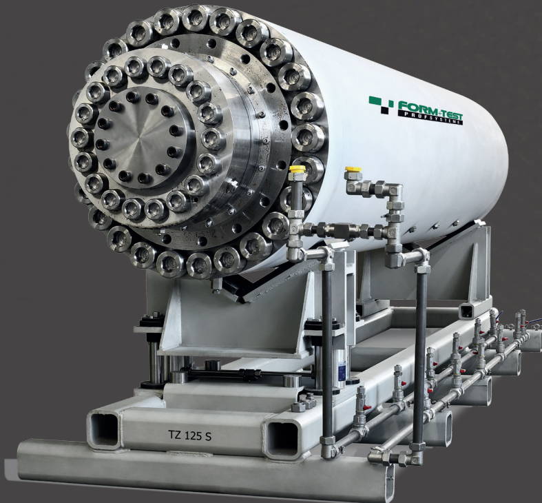
Pressure cell with 3000 mm of length and 125 MPa of pressure
