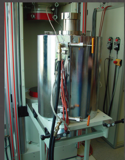
Pressure cell with 150 MPa and oil heating system
